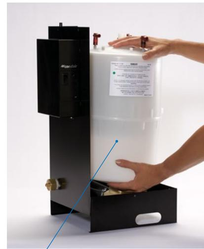
All scale and mineral sediment is deposited into the cylinders which are easily changed and discarded. Cylinder replacement requires no special tools and can be done in a few minutes.
